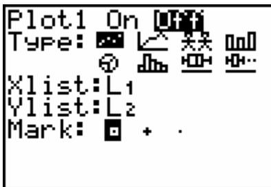
7. Using the cursor keys and **ENTER**, select **Plot 1 On**, **Type Line Plot**, **Xlist L1**, and **Ylist L2**.
